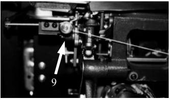
Pull twine to right side of machine. While gently pulling the stringholder release lever, place the twine under stringholder button # 9. Pull twine up and over button shaft and release stringholder release lever. Pull the twine taunt to cut off excess twine.
